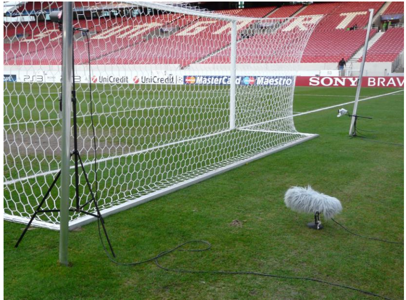
Typical setup of shotgun microphones on small stands at the edge of the playing field, in basket-type windscreens (see soccer arena graphic below)
